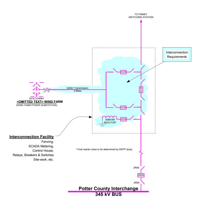
Figure 1, One-line Diagram of the 345 kV Interconnection Facility.
